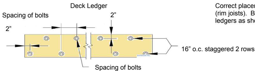
Correct placement of fasteners in deck ledgers (rim joists). Bolts must be placed in the deck ledgers as shown.
